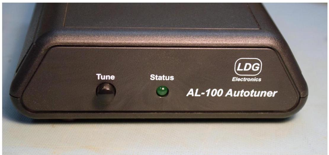
On the front panel there is one pushbutton and one LED indicator light.
